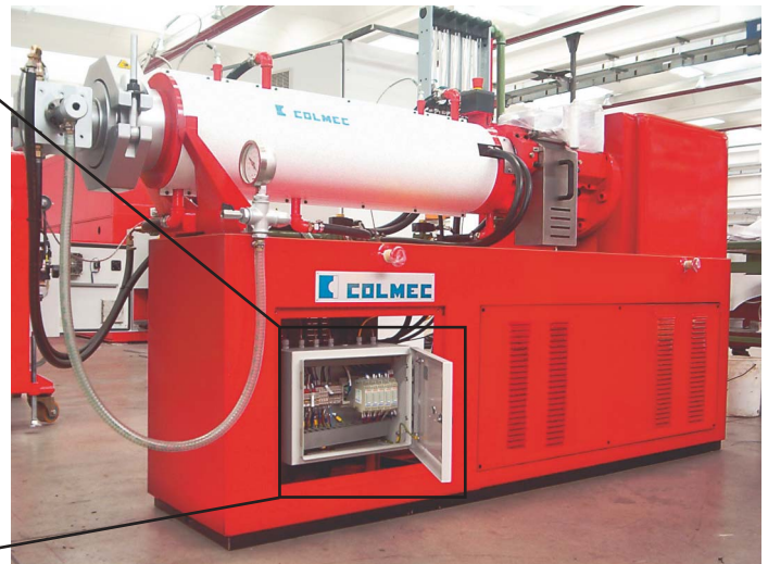
COLMEC extrusion line with Siemens PLC. Control and data acquisition are made by using delta due series (D1, D8 and D9). A gateway DX 5370 is installed to perform PROFIBUS-Modbus RTU data exchange and manager function for 16 instruments.
