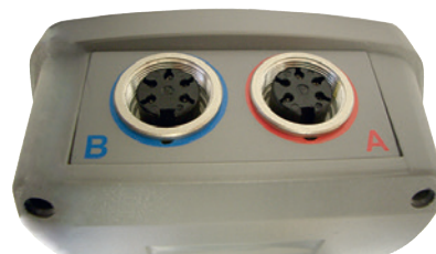
2 connection port for temperature probe inputs
